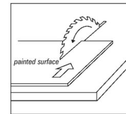
Normally a table saw's blade rotation is down. If this is the case, cut panel with painted surface face up. If blade rotation is up, cut panel with painted surface face down.
