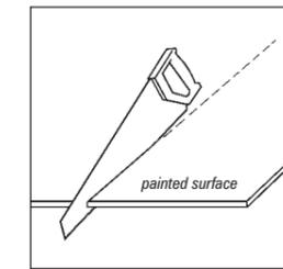
A fine tooth panel saw may be used to cut Seratone Oxides.
