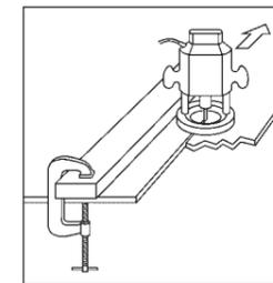
A router can be used to cut the panel, or alternatively, to finish an edge after cutting with a circular saw.
