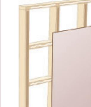
Apply at 400 mm centres on back of panel if mounting on existing wall lining
