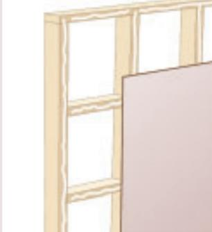
Apply at 400 mm centres on back of panel if mounting on existing wall lining
