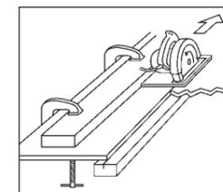
Normally the blade rotation of a circular saw is up. If this is the case, cut panel with painted surface face down. If blade rotation is down, cut panel with painted surface face up.
