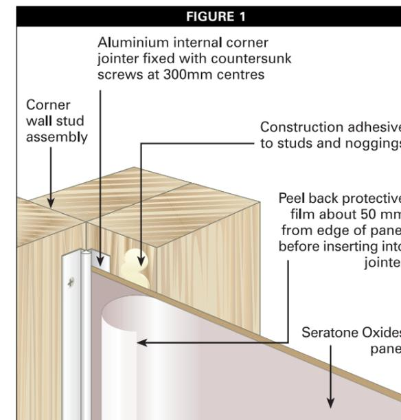
Continue installing by inserting each new panel into the jointer of the previous panel. Screw fix or glue jointers to studs as you go.
